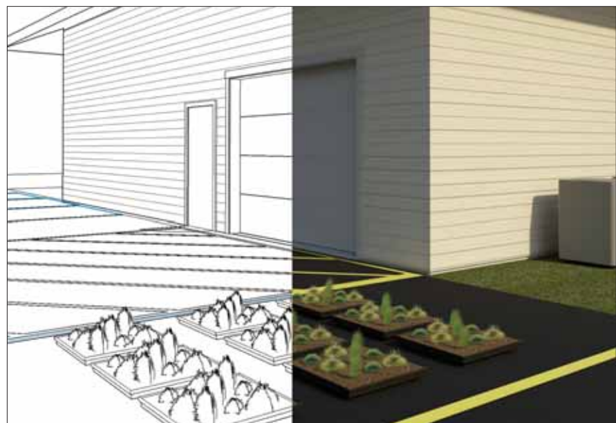
Figure Three. Using the model in this figure, a simple grid of Green roofing trays is placed in the parking lot. Obviously, they don't belong in the parking lot, but the figure shows the capability and power of current BIM packages. Both sides of this figure use the same camera location. The left half of the figure is what is seen while designing in real time, while the right half is a fully rendered version with shadows and textures. The ability to render images is built into many BIM packages.
