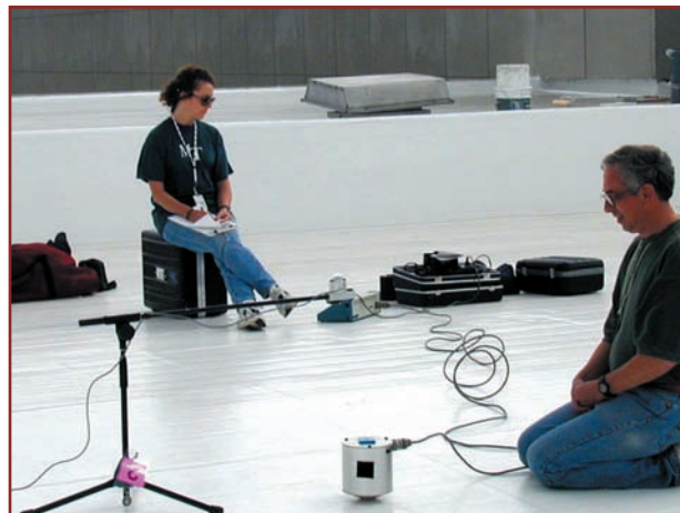
Photo 1: The microphone stand attached to a small meter (off camera) measures reflectance. The instrument which appears to be a gallon paint can attached by wire to a small suitcase is performing the D&S test.
