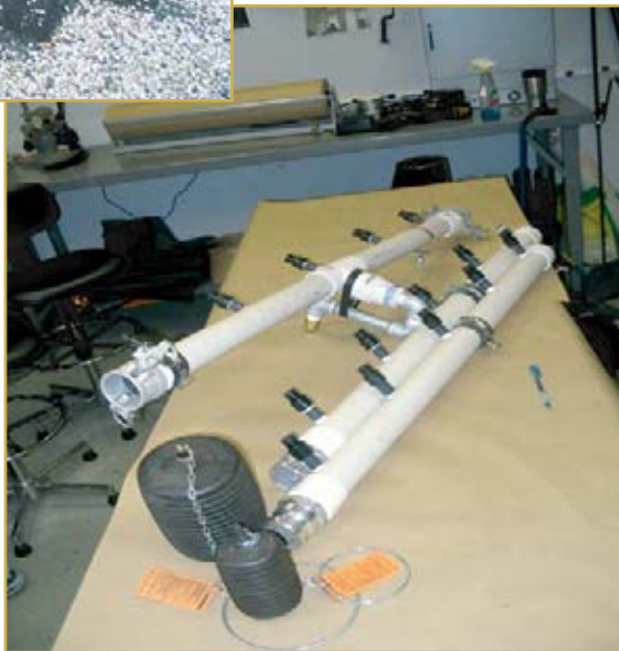
Photo 10 – Tools of the trade: shop-made spray bar and pneumatic drain plugs.
