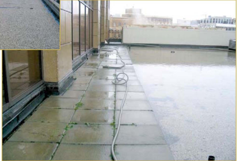
Below: Photo 6 – “Head of water” test on involved roof area.
