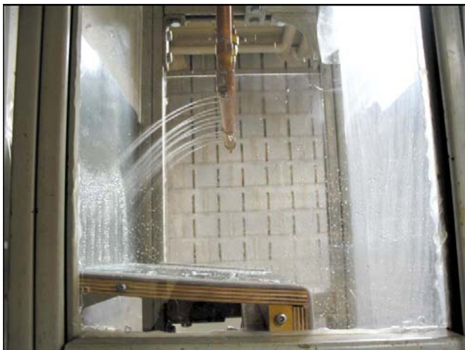
Figure 4 - Water being sprayed at the test specimen (flashing flatness in the test assembly was ensured during installation by fastening).
