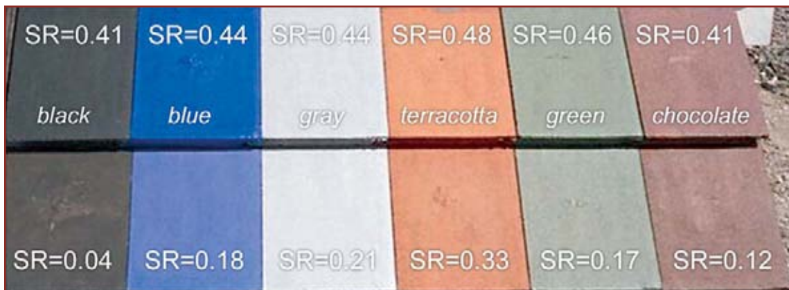
Figure 1 – Cooltile IR Coatings™ developed by American Rooftile Coatings and LBNL increase the solar reflectance of coated tiles by as much as 0.37 (black tile) without changing color.
