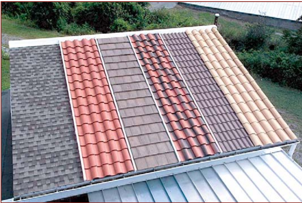
Figure 2 – An assembly of steep-slope attics was placed on top of the ESRA. Clay and concrete tiles were installed by the Tile Roofing Institute.
