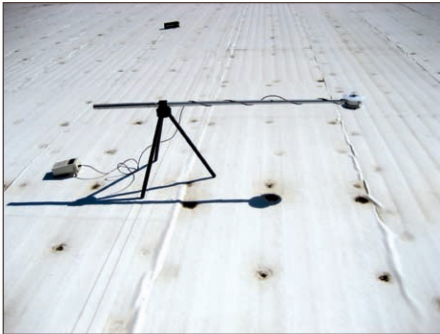
Photo 2 – EPDM in Minnesota, 1.5 years old, acrylic coating.
