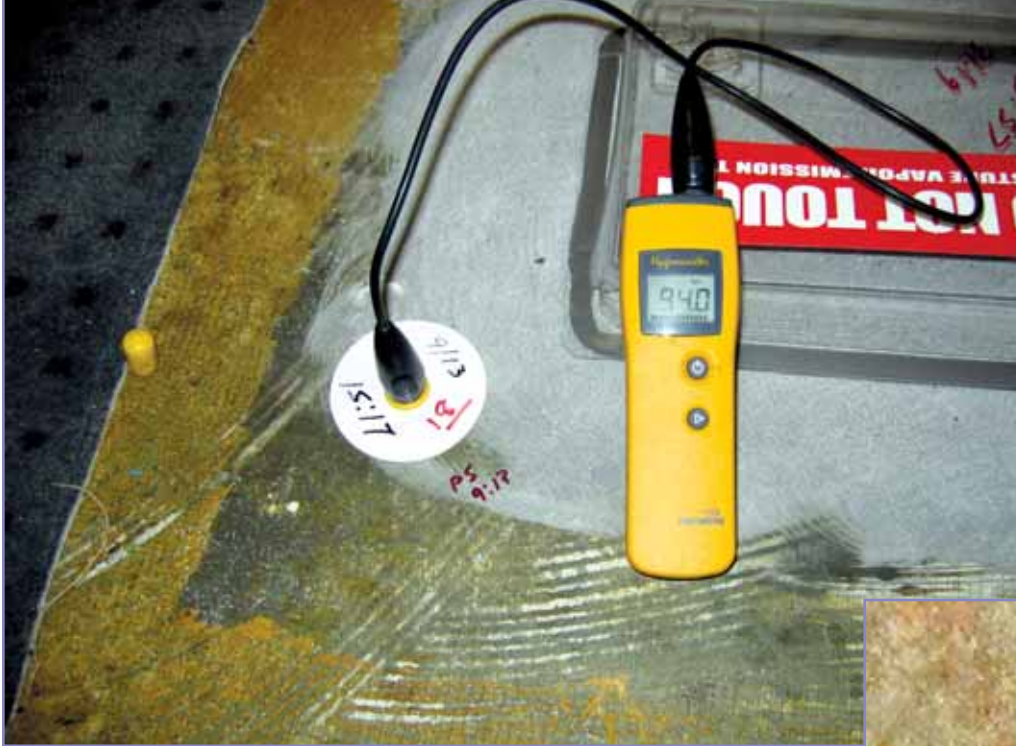
Concrete internal relative humidity (RH) test
