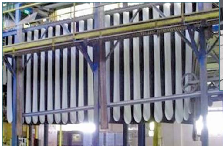
Bituminous products going through a factory-applied coatings line.
