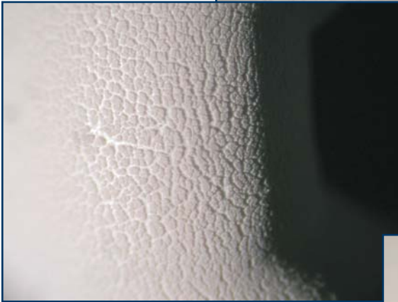
Photo 7 – PVC membrane #3 (14,000 hours).
