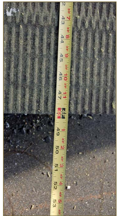
Photo 8 – Dimensionally stable stone wool arrived on site with exact dimensions.
