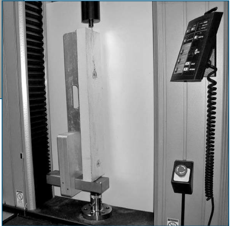
Photo 2 – Test setup of fastener with foam.
