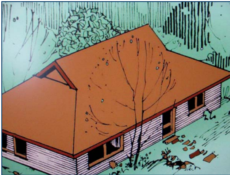
Figure 5 – Potential solution for hip roof ventilation.
